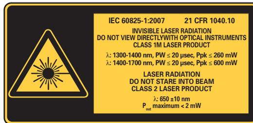
**CAUTION:** VIEWING THE LASER OUTPUT WITH CERTAIN OPTICAL INSTRUMENTS (FOR EXAMPLE: EYE LOUPES, MAGNIFIERS AND MICROSCOPES) WITHIN A DISTANCE OF 100 MM MAY POSE AN EYE HAZARD.
